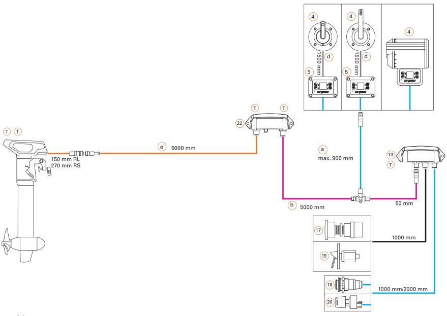
Bus system termination resistor
